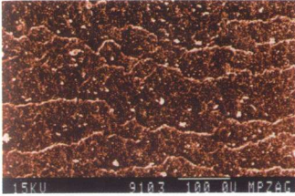
Surface image of the cot by electron microscope
