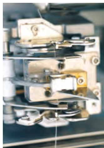
Convenient module system for material-adapted splicing.
