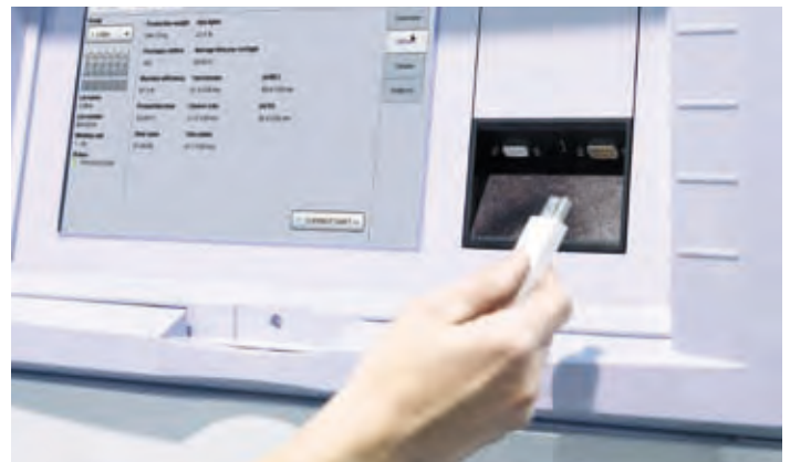
In addition to the 30 lots that can be stored in the Informator: external data storage and transfer via USB stick for quality that can be reproduced at any time and quick set-up
