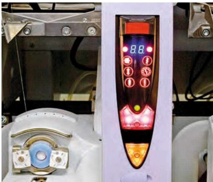
The winding unit display communicates in an easy to understand way. Symbols, pictograms and number codes help staff to make a targeted diagnosis
